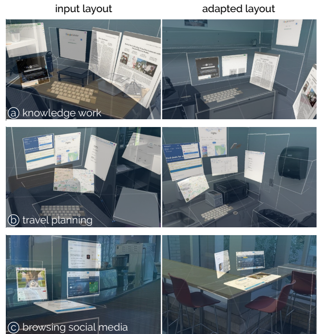
Figure 7: Possible use cases for InteractionAdapt : (a) searching for research literature, (b) planning a vacation, and (c) browsing social media. Left: Manually created layouts. Right: Layouts adapted by InteractionAdapt .
